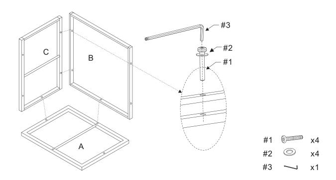
Step 2.Attach remaining side panel (part #B) to the assembled parts (part #A, B & C) using bolts (part #1), washers (part #2) and allen key (part #3). Attach remaining end panel (part #C) to the assembled parts (part #A, Bx2 & C) using bolts (part #1), washers (part #2) and allen key (part #3).
