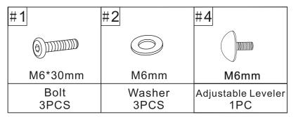
Step 1.Lay wicker top(part #A)on a flat surface with underside facing up.Attach one side panel (part #B) to the wicker top (part #A) using bolts (part #1), washers (part #2) and allen key (part #3). Attach one end panel (part #C) to the assembled parts (part #A & B) using bolts (part #1), washers (part #2) and allen key (part #3).
